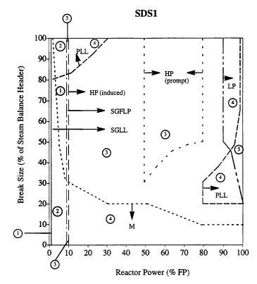
SGLL Steam Generator Low Level (conditioned out at 1% FP)
